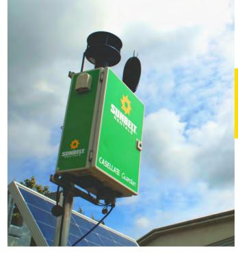
The unit will generate a multiple-format report on a schedule assigned by the user. The Guardian will also email or SMS alert users, in real-time, should any preset levels be exceeded. Guardians can be powered by a 110 – 240Vac, 12Vdc battery, a combination of both (for generator-powered sites) or a stand-alone solar option.
